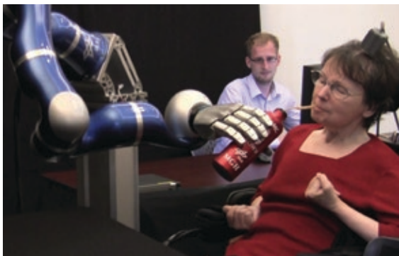
Figure 1. BrainGate2 clinical trial participant neurally controlling a robotic arm to give herself a drink of coffee, more than 14 years after becoming tetraplegic and anarthric from a pontine infarction (Hochberg et al., 2012). Caution: Investigational device. Limited by federal law to investigational use.
